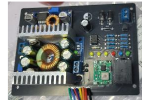
Power distribution board
